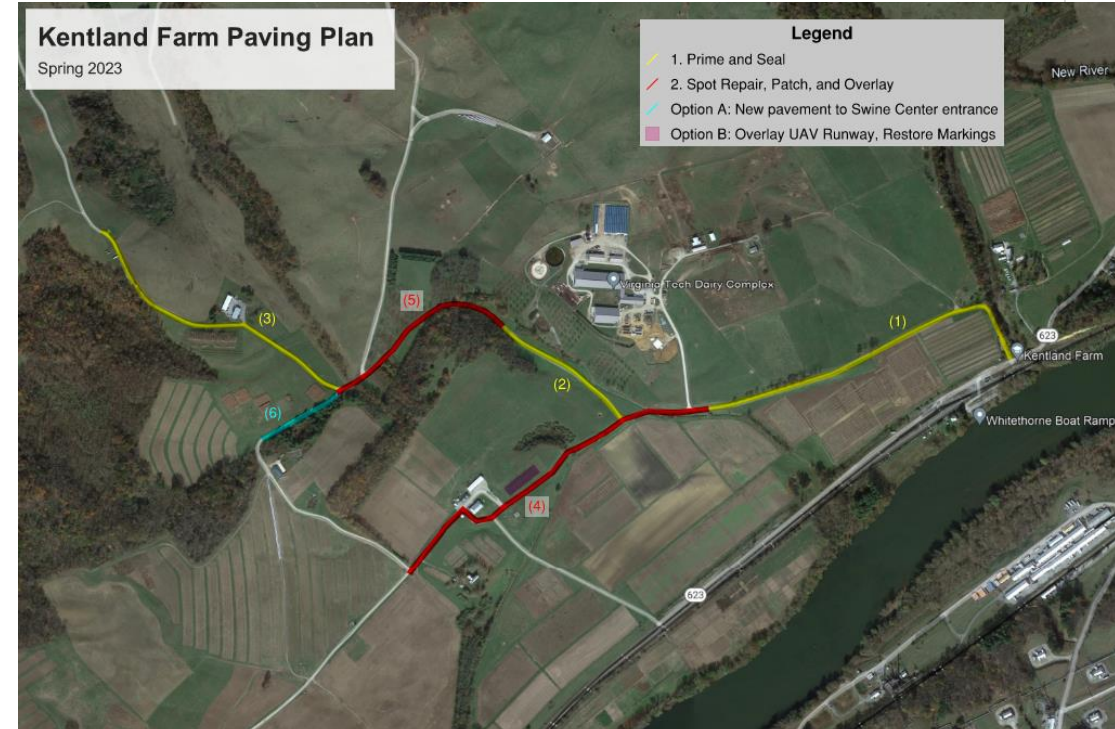
Kentland Farm Roadway Maintenance and Repaving
